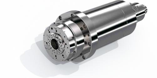
The self-developed HSK E40/HSK A63/HSK A100 built-in spindle. Eliminates jitter and vibration in the range of spindle rotation, and achieves stable accuracy in high-speed long-time machining. The spindle uses forced cooling to cool the motor and front and rear bearings.
